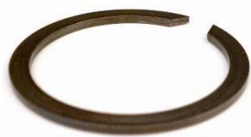
Gates Part # SR144 Thickness: 1.44mm End Detail: Angled, w/ Gap
