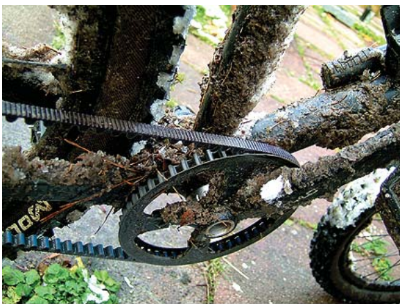
The mud-shedding design of Gates Carbon Drive™ System includes a chainring with patented Mud Ports™ that keep the drive clean and fully functional even in conditions that tear traditional bicycle drivetrains to pieces.
